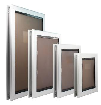
Designed to be aesthetically pleasing whilst maintaining the rugged durability of aluminium construction. Suitable for dual glazing installations with an additional glazing kit. The door will fit an IGU unit with a thickness between 18mm to 40mm. Flexible unbreakable flaps seal against the aluminum frame with a brush weather seal, held in place by powerful magnets. Ultimate security is provided via a tough composite panel with a robust locking mechanism.
